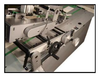
Adjustment knobs quickly and accurately set feeder location and height.
