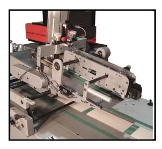
Pivot the feeder upward and away from the transport table for jams or maintenance.
